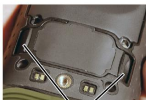
Grasp SD Card door edges and pull
